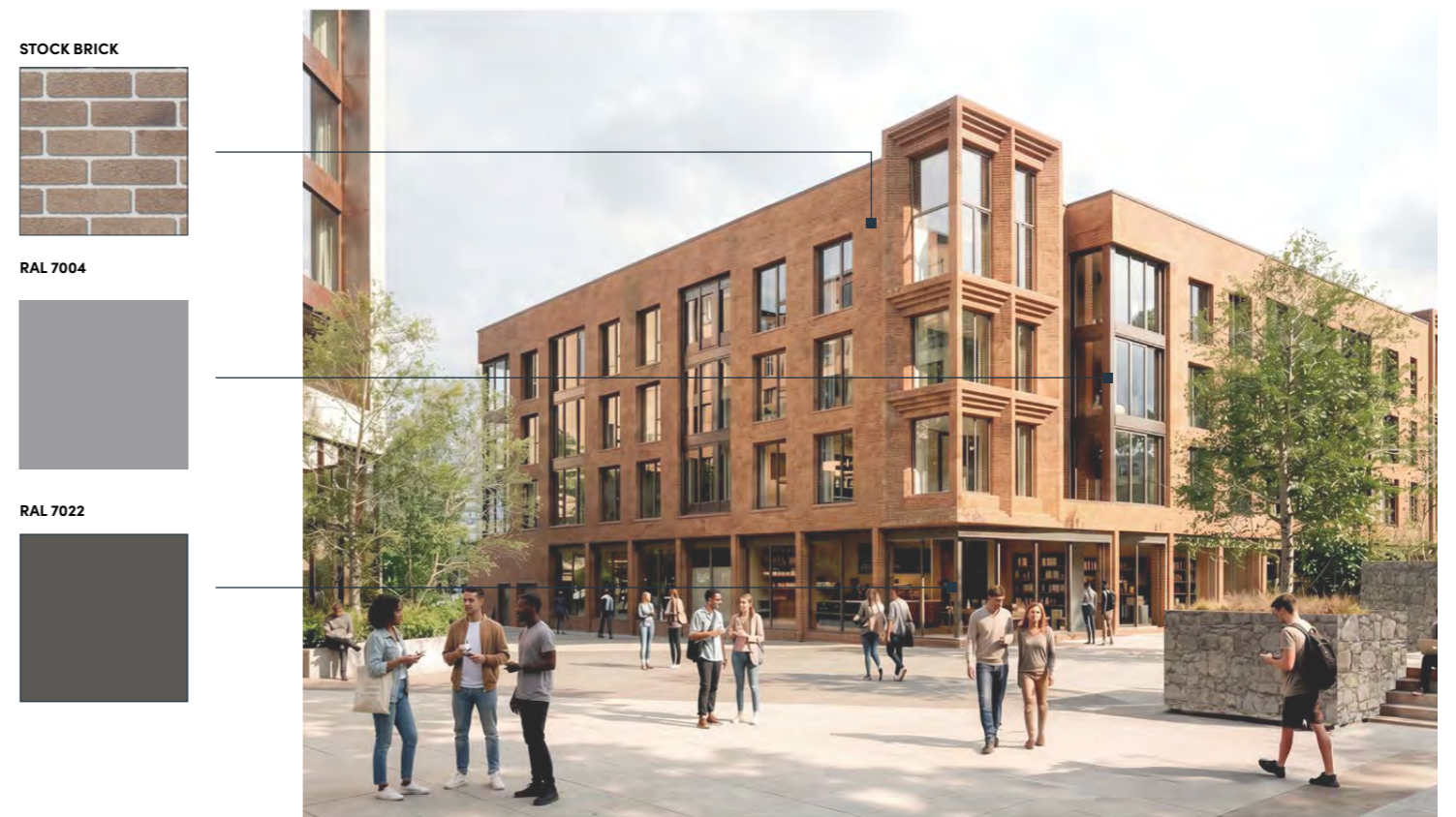
Figure 6-15. CGIs of new blocks proposed (Student Accommodation and mixed-use block) highlighting their principal materials. Source: MCORM, 2026.
